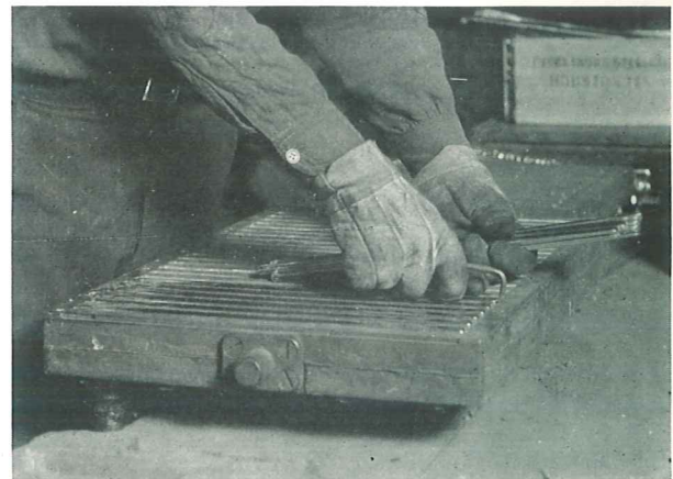
Above: Solder being cast into bars. Below: Bars being removed from mold. Imperfect bars are discarded.
