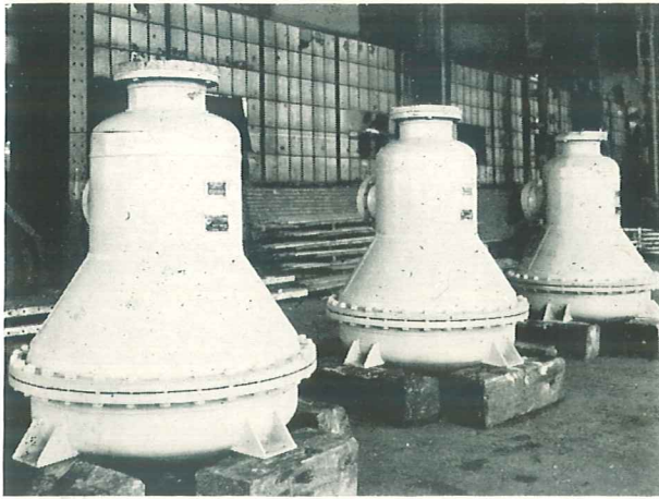
Above: Three homogeneous lead-lined steam separators. Below: Lead-lined steam jacketed steel drum.
