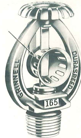
Sprinkler head controlled by fusible alloy. Arrow points to soldered joint.
