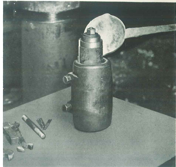
Pouring a babbitt lining. This method, used in many machine shops, is usually employed for the smaller bearings.
