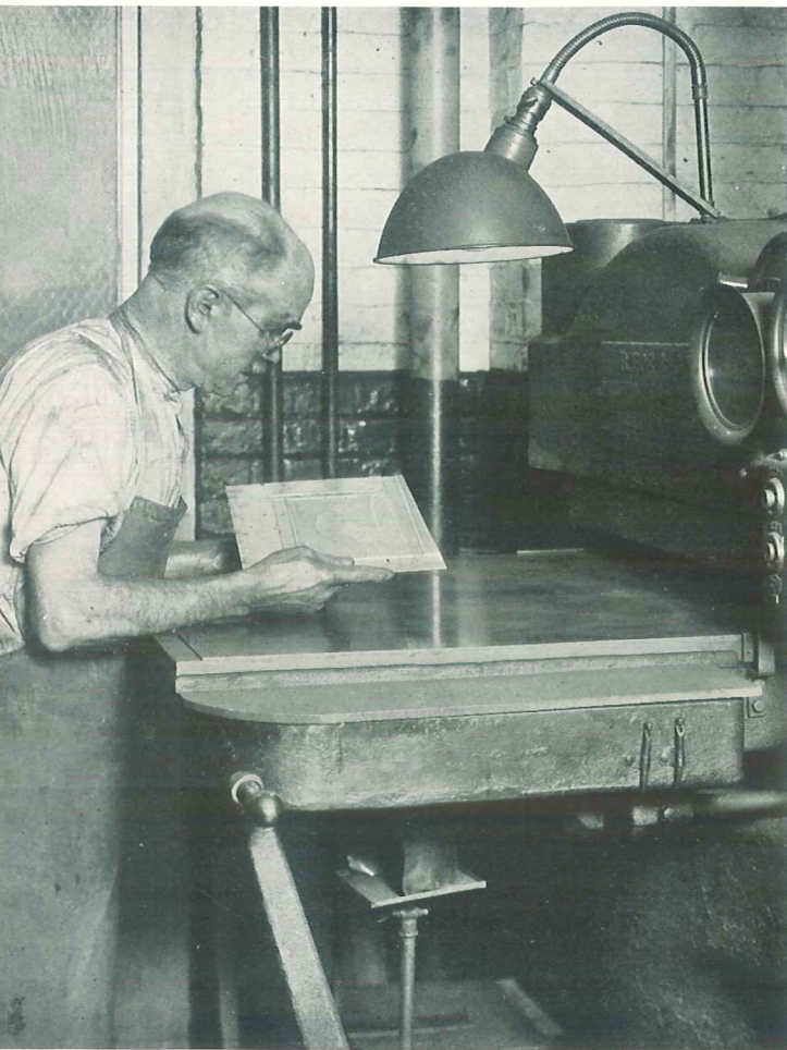
Molding press for use in molding impression lead.
