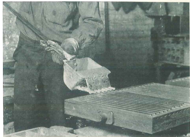
Above: Solder being cast into bars. Below: Bars being removed from mold. Imperfect bars are discarded.
